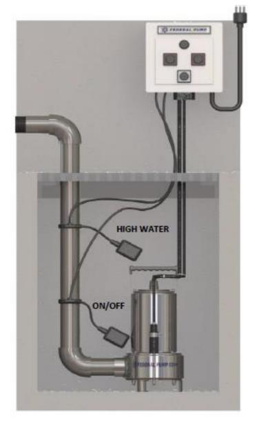
the event of presence of oil, the oil sensing element will terminate pump operation and sound the alarm horn and light alerting the presence of oil in the sump.
