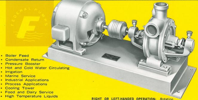
**CAPACITY:** From 1 to 150 GPM against heads up to 550 ft. Capacity varies only slightly even if there is considerable variation in the head condition. Capacity can be increased or decreased by changing cover plates and impeller.
